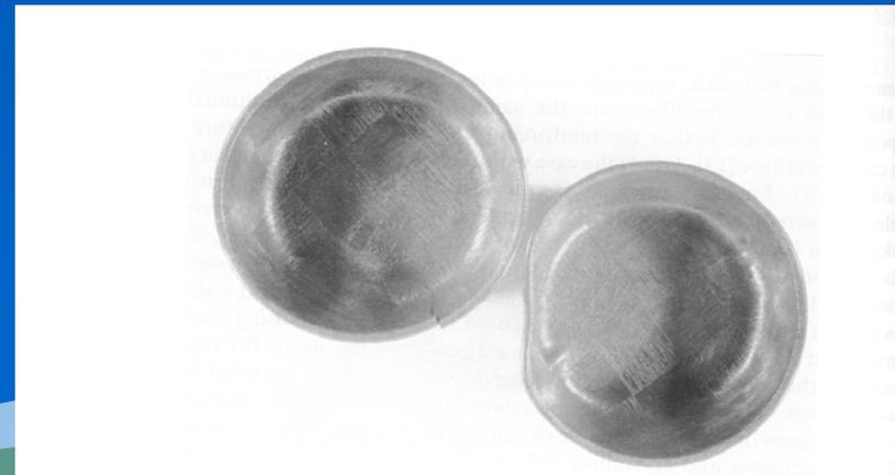
Figure 6-8 IPS salad bowls deformed and cracked due to washing in dishwasher
