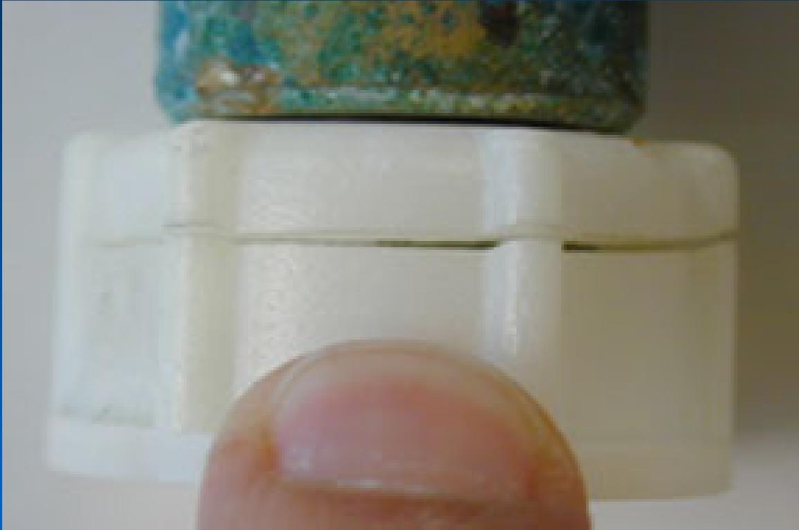
**Failure resulting from ignoring installation instructions**
