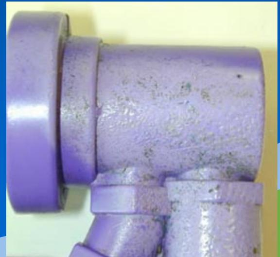
Degradation from prolonged contact with Gasoline
