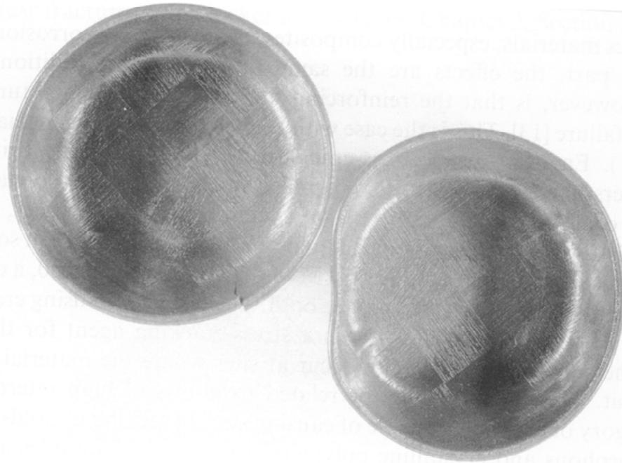
Figure 6-8 IPS salad bowls deformed and cracked due to washing in dishwasher
